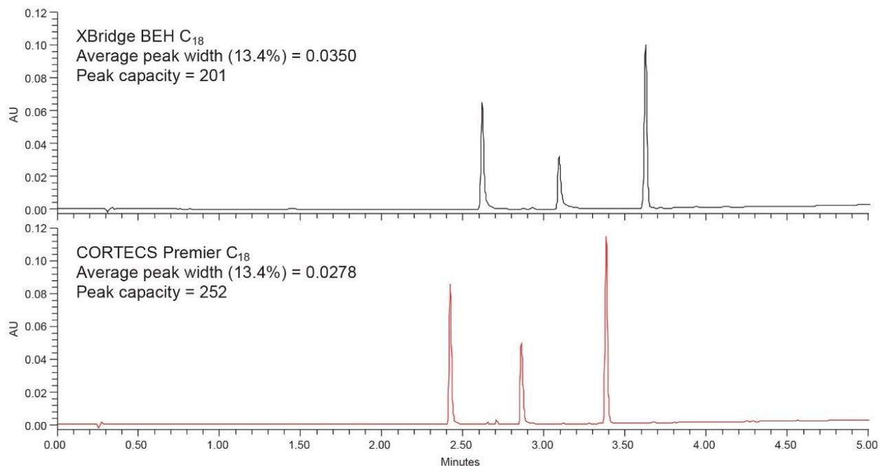
Figure 4. Separation of three analytes using XBridge BEH C<sub>18</sub> XP and CORTECS Premier C<sub>18</sub> Columns. Calculated peak capacity is shown. 1) Fostemsavir, 2) Betamethasone Phosphate, 3) Betamethasone.
