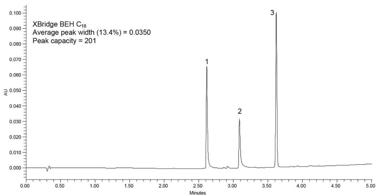
Figure 2. Separation of three analytes using the XBridge BEH C<sub>18</sub> XP Column. Calculated peak capacity is shown.
