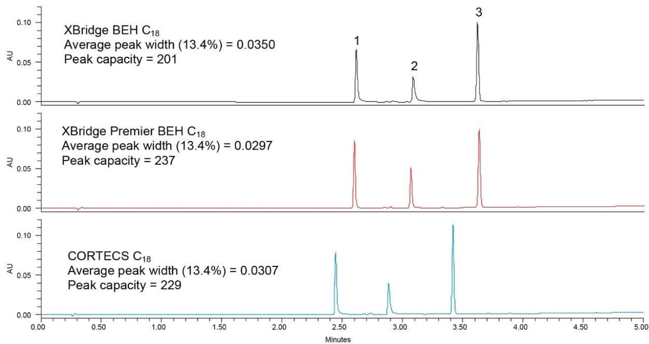
Figure 3. Separation of three analytes using XBridge BEH C<sub>18</sub> XP, XBridge Premier BEH C<sub>18</sub>, and CORTECS C<sub>18</sub> columns. Calculated peak capacity is shown. 1) Fostemsavir, 2) Betamethasone Phosphate, 3) Betamethasone.
