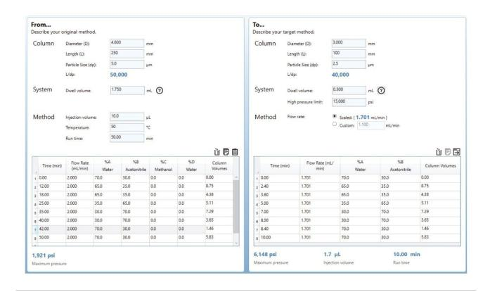
Figure 4. Waters Columns Calculator used to scale down a method from a 4.6 x 250 mm, 5  $\mu$ m column to a 3.0 x 100 mm, 2.5  $\mu$ m column.
