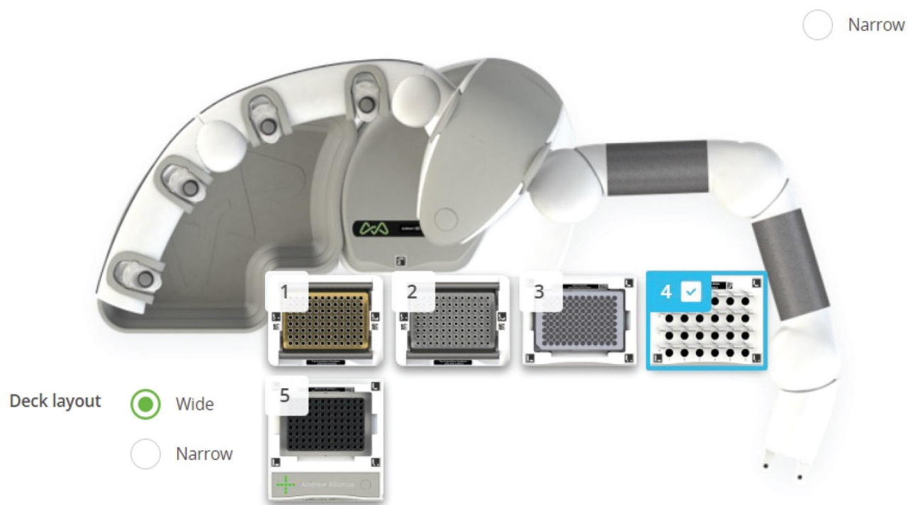
Figure 2. Andrew+ Deck Layout for sample preparation of standards and samples using Andrew+ Pipettes and Domino Blocks: 1. Tip insertion system (5-120 µL Optifit tips); 2. Tip insertion system (0.2-10 µL Optifit tips); 3. Microplate; 4. Microtube; and 5. 96-PCR Plate Peltier+.
