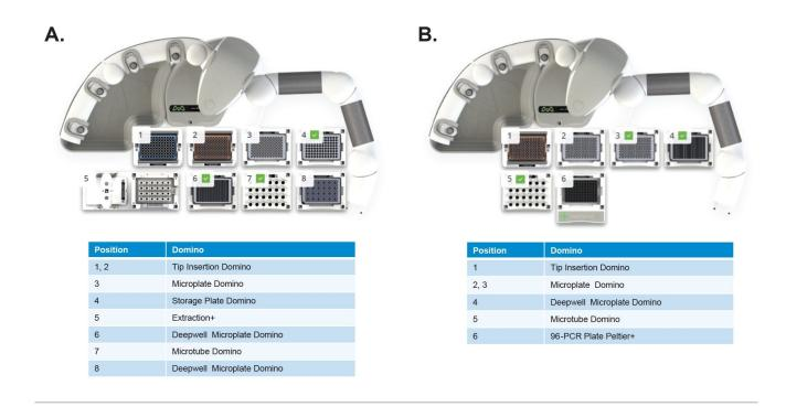
Figure 3. Deck layouts for the 24-sample automated PeptideWorks workflow. Protocol A executes denaturation, reduction, and alkylation and protocol B executes concentration normalization and digestion.
