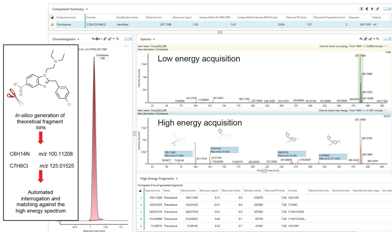
Figure 5. Tentative detection of clonitazene in a mixed benzimidazole (nitazene) opiate standard sample by screening using a Molfile. This class of synthetic opioids can exhibit potency up to several hundred times that of morphine. In this sample, the processing highlighted an unknown peak with a mass of m/z 387.1588. In-silico fragmentation is automatically performed for all Molfiles added to the library and yields theoretical fragments which are then sought in the high energy MS E data. The tentative detection of clonitazene was subsequently confirmed following analysis of CRM.
