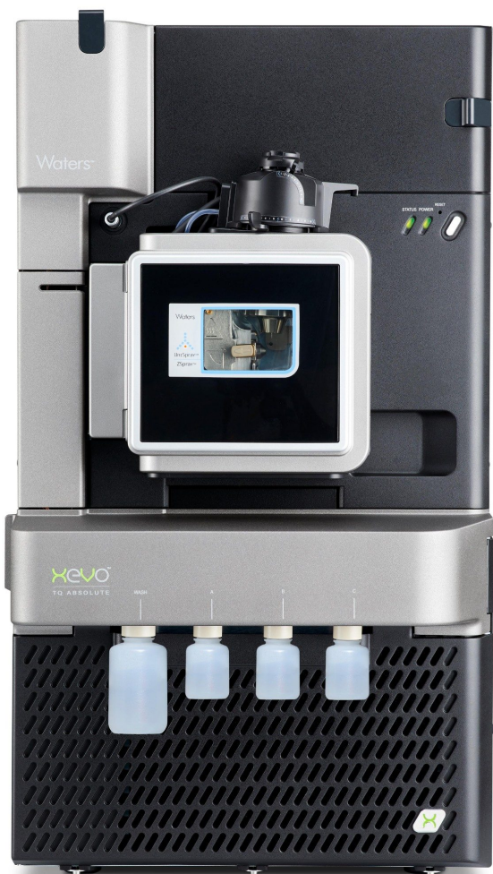
Figure 1. Xevo TQ Absolute Mass Spectrometer.
