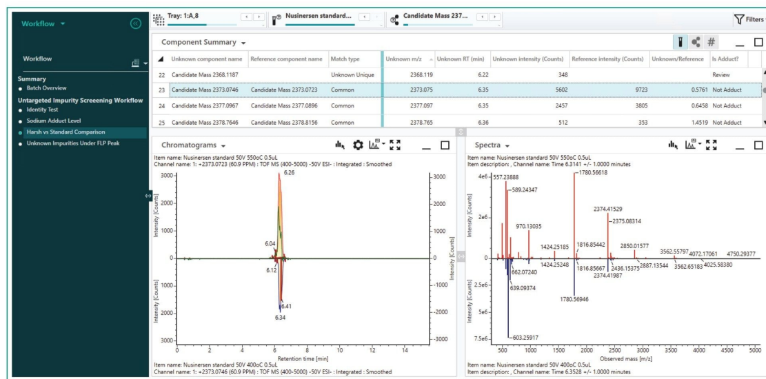
Figure 7. Guided data review workflow step comparing harsh versus soft ionization for distinguishing adducts from impurity peaks of the same m/z using mirror plots in the Untargeted Workflow.
