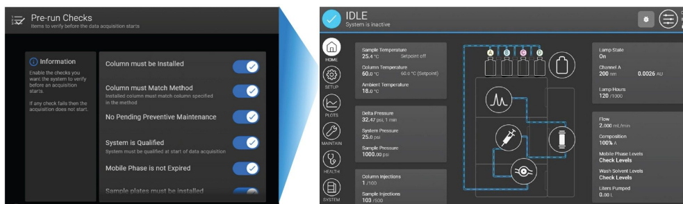
Figure 4. The pre-run configurable checklist can be found in “setup” on the Alliance iS Bio HPLC System touchscreen interface.
